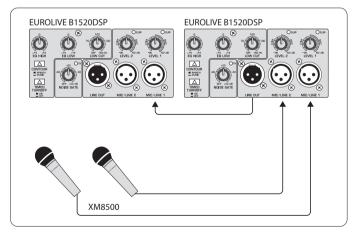
Fig. 4.1: Connecting microphones
